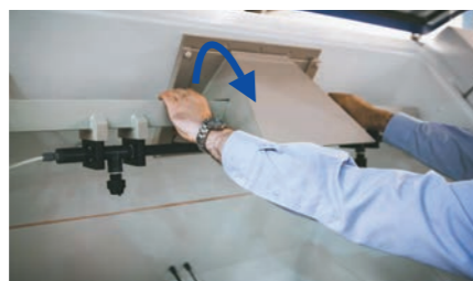
2. The combined air dispersal and oscillating spray bar unit simply lifts out.
