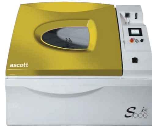
Standard 1000 Ltr salt spray chamber
