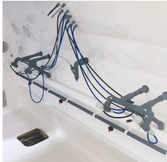
Example of dual atomiser system on 2600L Atmosfär Premium Chamber
