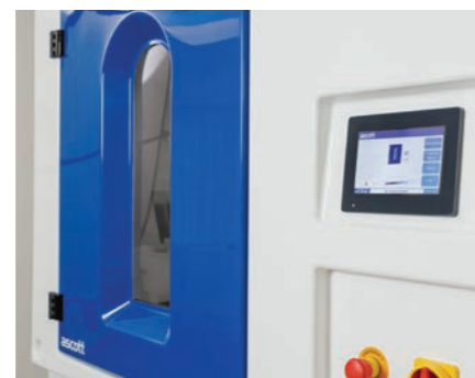
KH300 Control panel and window canopy
