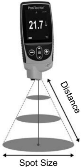
The distance to spot ratio refers to the relationship between the diameter of the area being measured compared to the instrument's distance from the area. As the distance (D) from the target increases, the spot size (S) of the area being measured by the unit becomes larger. The D:S ratio of the **PosiTector IRT** is 5.7:1. For example, when the instrument is 100 cm (40 inches) from the target, the spot size will be about 18 cm (7 inches) in diameter.
