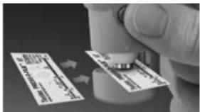
To position the tape, align the two dots (printed on replica tape) with arrows on both sides of the measurement opening.
