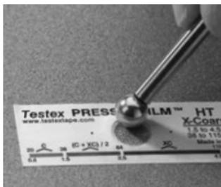
Apply replica tape to blasted surface. Press the adhesive-backed ends of the tape to hold it firmly in place during the burnishing process.
