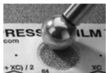
Firmly compress the foam using the rounded end of the included stainless steel burnishing tool. Apply sufficient pressure in a circular and x-y rubbing motion to produce a replica with a
