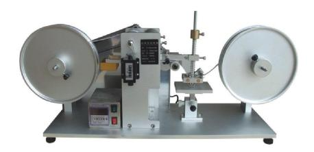
R.C.A Paper Abrasion Wear Testers make it simple to test smaller areas such as keypads for abrasion. The design also makes it easy to test curved, convex, and concave surfaces.
