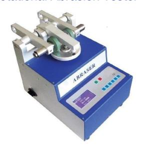
Rotational Abrasion Tester determines the abrasion resistance performance of various coatings as well as paper, plastic, textile fabric, etc.
