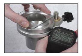
8. Watch the flow of liquid from the orifice and stop the stopwatch the moment the flow breaks.
