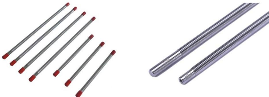
Traditional wire bar coaters are not suitable for ultra-thin coating, in addition to this, the fine wire on the surface can be easily broken, and they can be difficult to clean. To overcome these issues, we recommend Wire Formed Rods. CNC machined with precision moulding, the deviation of the groove depth and space is lower than  $2\mu\text{m}$ , giving a uniform film application
