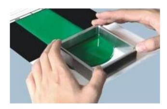
The square film or Octoplex applicator has eight predefined thickness sides for flexibility. It is manufactured from high-grade, corrosion-resistant stainless steel
