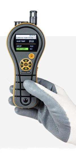
The steel surface temperature generally should be at least 3°C above the dew point when paints are applied. Below this temperature the Dewpoint Meter will sound an alarm and the display colour will change to warn you that the surface conditions are not suitable to paint.
