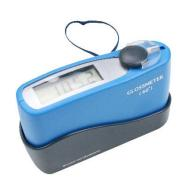
This Basic Glossmeter has a plastic shell and one-body standard board. It can be used for many different applications paints, film, ink, plastics etc. It is compact, easy to use and takes a single AA size battery.
