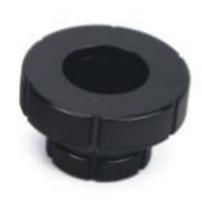
Perme cups are used to determine the permeability of films to the vapor of water and other liquids. Materials that are tested include paint, varnish, thin plastic films and other types of sheets thin enough to be tightly sealed in place across the face of the cup.
