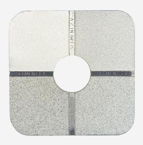
When steel has been blast-cleaned, the surface consists of random irregularities with peaks and valleys that are not easily characterised.
