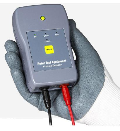
Connect the Earth Cable to the base metal of the item under test. It is essential that the base metal of the item being tested is also connected to a true earth.
