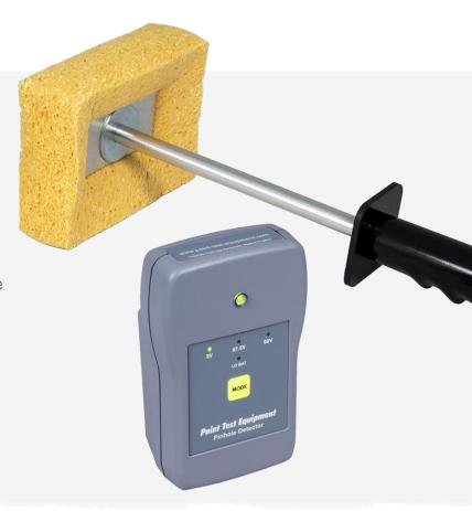
Operation is by a wet sponge, moistened with a wetting agent, being moved over the coating. The wetting agent penetrates any pinhole and makes a conductive path through to the substrate.
