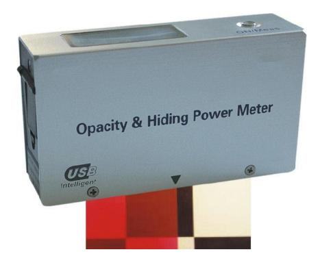
This opacity meter is used to measure the opacity, or luminous reflectance, of a grey scale. Suitable for the evaluation of a coatings hiding power, or simple shade sorting tasks of metallized films, anodised aluminium, or ceramics. It can calculate the contrast ratio (opacity) and store it.
