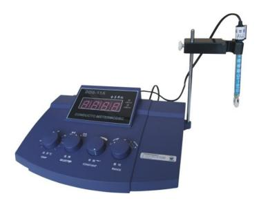
Table mounted conductivity meter with large back lit LCD screen which displays conductivity temperature values, with manual or automatic temperature compensation. It has four types of electrodes for conduction cell constant: 0.01,0.1,1.0 and 10.0cm-1.
