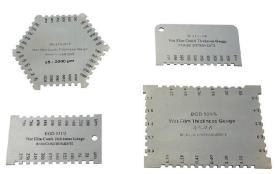
Our Wet Film Thickness Gauges have a comb-shaped design with precision cut gaps to determine the coating thickness by placing vertically onto a wet coated substrate.
