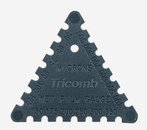
Manufactured in Plastic, the Wet Film Gauges can either be kept as a record for the wet film thickness taken or cleaned in solvents and reused.
