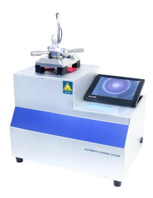
The punch on this Automatic Cupping Tester can rise automatically at the speed of 0.2mm/s as required by some standards. This eliminates errors caused by hand lifting.
