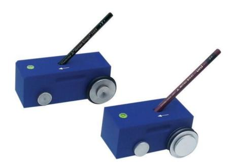
This instrument offers an easy method for the determination of film hardness for coating applied to a flat substrate. The pencil lead, prepared beforehand by rubbing it on fine abrasive paper (400), is maintained at an angle of 45° and pushed with uniform pressure onto the sample, either leaving a superficial trace or causing destruction down to the substrate. It complies with the requirements of ASTM D 3363, ISO 15184.
