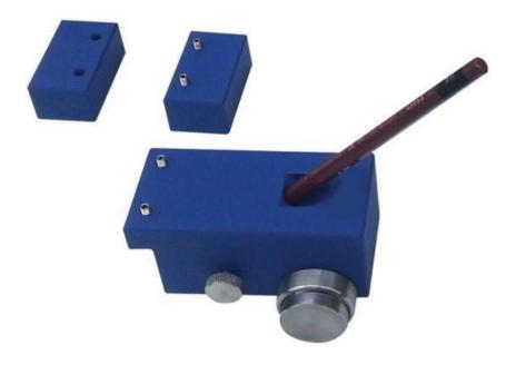
Our Adjustable Pencil Hardness Tester is designed in accordance with ASTM D 3363 and ISO 15184.lt enables the user to obtain three different weights (500g,750g and 1000g) by selecting a different loading weight.
