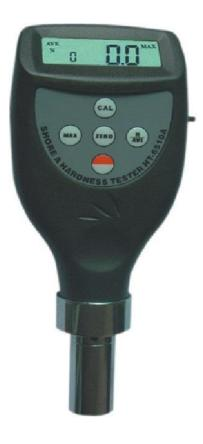
Compact Shore Hardness Meter with an integrated probe. With RS 232 interface and auto switch off. Displays hardness result, average value, max. value. Relevant Standards: DIN53505, ASTMD2240, ISO7619, JISK7215
