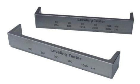
The Levelling Tester is designed to determine the relative levelling of liquid coating materials before curing in the laboratory. (Coating materials have to eliminate surface defect during drying). It complies with ASTM D2801-1994 (T01-700133) and NYPC (T01-700134)
