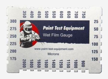
Manufactured in aluminium, the Wet Film Gauge can either be kept has a record for the wet film thickness taken or cleaned in solvents and reused.
