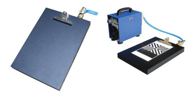
Vacuum plates are made of aluminium and finished with an anodized grey hard coat giving high corrosion resistance, improving the longevity of the vacuum plate. The top section of the plate has a series of holes. When connected to a vacuum pump or sink aspirator, the vacuum suction created keeps the paper charts in place.
