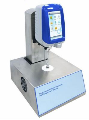
The Programmable Touch-Screen Viscometer with Temperature Control combines viscosity measurement and temperature control in one machine. This removes the need for a separate thermostatic bath, viscometer, and small sample adapter.
