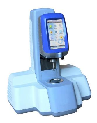
The Cone and Plate Viscometer is used to test the dynamic viscosity for non-Newtonian fluids, (paint and surface coatings). The Cone and Plate Viscometer is used to reflect the real-life representation of typical changes of paint when applied with a roller, brush, or spray gun under high shear rates.
