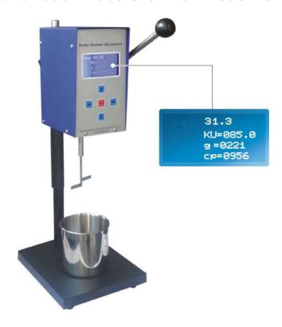
The Advanced Digital Krebs Viscometer is used widely for making viscosity measurements on paints/coatings in accordance with ASTM D562. Digital version with constant speed motor rotating at 200 r. p. m to produce greater accuracy and repeatable test results. The same standard key features as the standard Krebs Viscometer (model ref T01-700334) but with additional advanced key features (See below)
