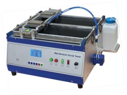
Our Wet Abrasion Scrub Testers can produce repeatable, controlled conditions to simulate everyday use or wear pattern and examine washability and related properties that affect the stain resistance of coating as well as determining detergent performance in a reproducible manner. We offer several options dependent on the test standards being followed
