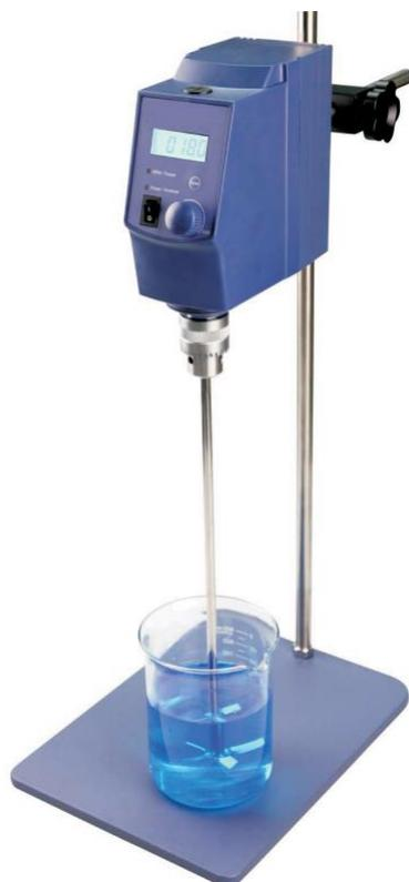
High quality precise digital overhead stirrers with brushless motor for smooth and reliable operation. Auto cut off for safety and capable of running for extended periods of time
