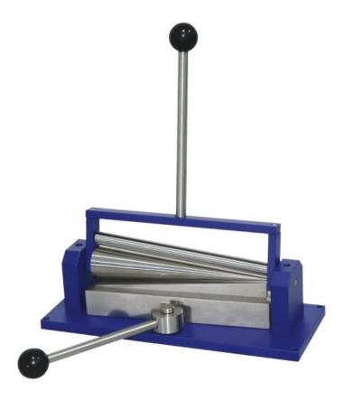
The Conical Mandrel Tester is used to determine the extensibility of paint coatings on metal panels that are clamped in position and formed round the conical mandrel by rotation of the roller frame. The panels are then examined to evaluate crack resistance and detachment from the metal substrate. This instrument allows easy identification of any coating failure at a specified diameter, over partial or entire mandrel length.
