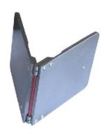
This Hinge-type Cylindrical Mandrel tester consists of eight hinges each with a different diameter axis. Place the test panels into hinge then fold to complete a 180° bend.
