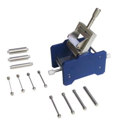
This Cylindrical Mandrel tester consists of three PVC rolls which are arranged side by side and run on pivoting bearings. Thus, the coating is not exposed to damage or shear stress during the test.
