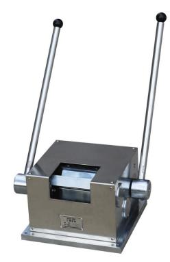
T-Bend Tester is designed to evaluate the flexibility and adhesion of an organic coating on a metallic substrate by observing the cracking or loss of adhesion when a coated test panel is bent. This method can be used to confirm whether paints, varnishes or related products meet a given test requirement in a pass/fail test, or to determine the minimum bending diameter at which cracking does not occur.
