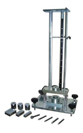
The DuPont Impact Tester has been designed to test the endurance of coated material, when impacted by a falling weight at specified points. The purpose of the test is to see if test specimens can resist the effect of rapid impact testing. The principle of the test is that a coated test specimen is impacted by a falling weight, at a fixed height; thus checking the damage or deformation of the test specimen.
