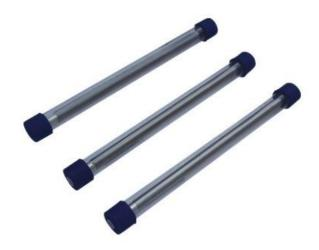
The wire-wound rods are made from stainless steel and are corrosion-resistant. A coating of paint or ink is drawn down by a known thickness wire-rod applicator over a substrate (e.g., Black/White Test Chart, Glass or Wood Panel, etc.) The motion of the drawdown is done by gripping the 2 edges of the applicator or by using the holder (available as an optional accessory)
