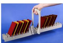
These sample racks comprise of three parallel slotted support rails, which are flexibly connected together in-line. The outer two rails are fixed and the centre rail is adjustable - using a hand operated lever. The inner rail can therefore be moved backwards/forwards with respect to the fixed outer rails
