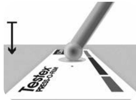
**NOTE:** The stick-type legacy burnishing tool remains a valid measurement practice and is recognized by international standards, but does not have an associated accuracy statement. See Accuracy (pg. 5).
