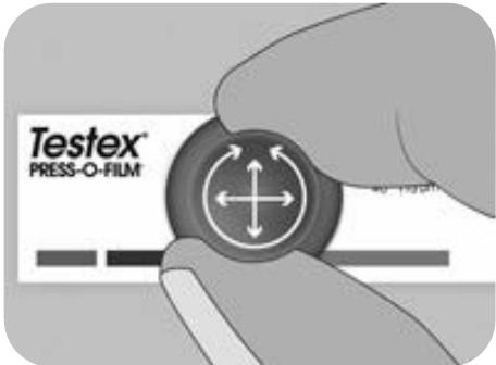
5. Alternate between linear (x-y) and circular motions with the burnishing tool to completely burnish the replica foam until a uniform stippled gray appearance is achieved across the entire measurement area.
