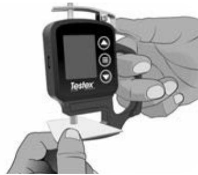
**NOTE:** Clean the anvils prior to turning on the gage, zeroing (pg. 6), or whenever the gage does not display -50 µm (-2.0 mils) when replica tape is removed after taking a measurement.
